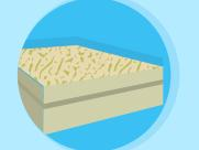
A ½ -pound-density urethane foam that fully insulates the space between the shell and the cabinet.
