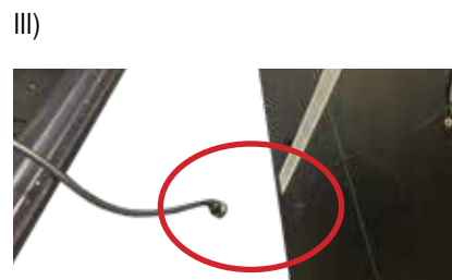
Using both hands grab wire on each side of connector and pull away from connector.
